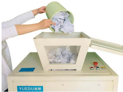
Fig. 3: Feeding View (Hopper with Auto-Lock)
