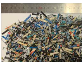
Card Shredding to 4mm Particles
